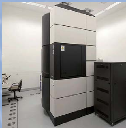
Figure 1: The aberration-corrected Titan 3 80–300 transmission electron microscope
